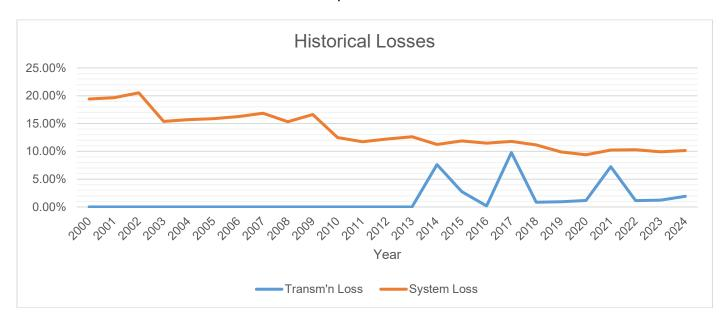
Historically, Transmission Loss ranged from 0.19% to 9.78% while System Loss ranged from 9.38% to 20.52%. Transmission Loss peaked at 9.78% on year 2017. System Loss peaked at 20.52% on year 2002 due to overloaded substation power transformer and centralized maintenance office.
